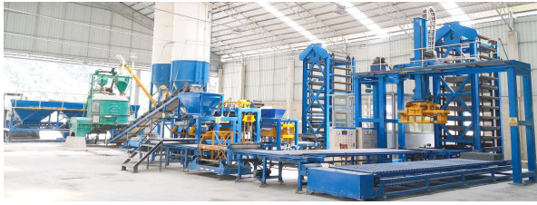
Full automatic concrete block manufacturing plant
