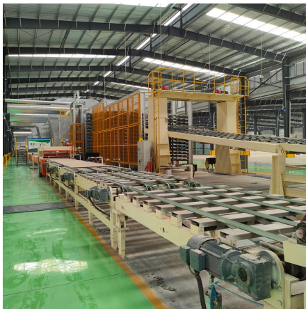
Automatic dryer discharge and roller conveyor
