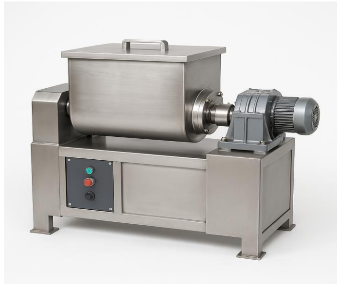
Sigma mixer used for blending soap noodles and additives
