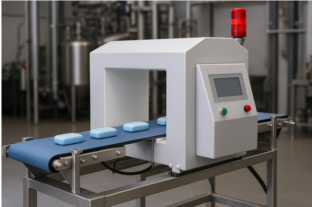
Metal detector scanning soap bars on conveyor
