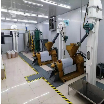
Supplier reference: real screw oil presses and feed elevators suitable for compact apricot-kernel oil extraction after trials.
