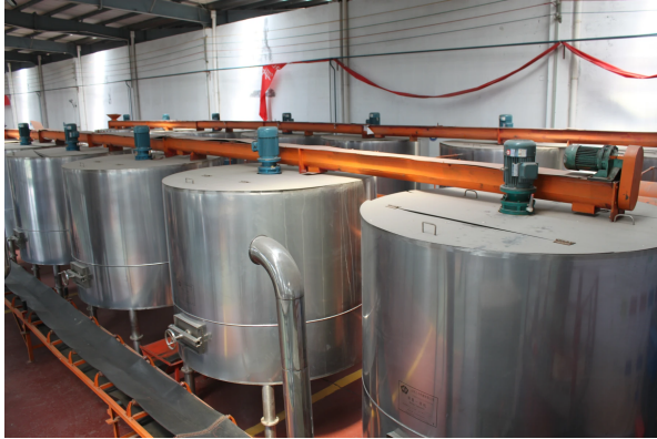
Supplier reference: real one-tonne-class stainless germination and kilning vessels for a small malt plant.
