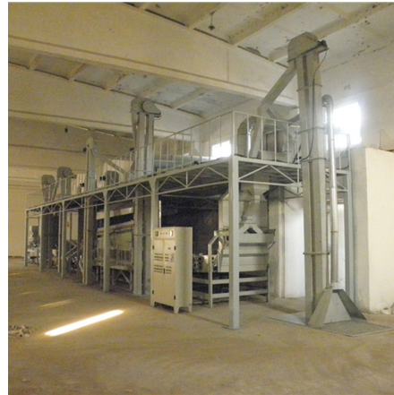
Supplier reference: real air-screen cleaner and grader suitable for configuration with lentil screens.
