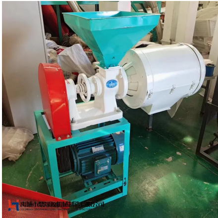
Supplier reference: compact maize peeling and milling machine for small-workshop output.
