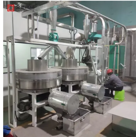
Supplier reference: multi-stone milling installation with enclosed flour transfer.
